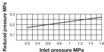
This chart shows variation in reduced pressure when the inlet pressure of 0.6 MPa is changed between 0.2 MPa and 1.6 MPa while the reduced pressure is set at 0.2 MPa.
