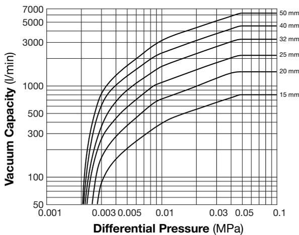
1. Differential pressure is the difference between the inlet pressure of the check valve and the internal pressure of the piping system.
