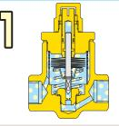
At startup, the bimetal element is contracted. The coil spring holds the valve open, quickly discharging the cold air and initial condensate.
