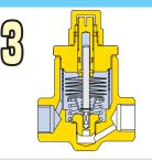
When the condensate reaches the preset temperature, the valve shuts tightly, stopping all condensate discharge.
