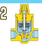
When the condensate temperature rises, the bimetal begins to expand. The valve begins to close, allowing less condensate to flow.
