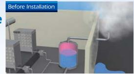
A condensate tank vented to atmosphere generates flash steam. Pressure cannot be applied to the tank, so conventional heat exchangers cannot be used.
