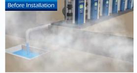
Boiler blowdown is hot and contains significant amounts of energy, however conventional heat exchangers are difficult to implement since they add back pressure to the boiler, therefore blowdown into a pit is more common.
