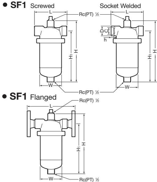
**SF1 Screwed\*/Socket Welded** (mm)
