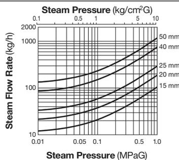
The chart to the left is used to determine the steam flow rate through the SF1 separator-filter. It is based on a steam velocity in the piping of 30 m/s. For other cases, use the equation below and replace "v" with your steam velocity:
