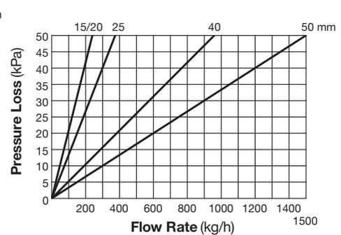
These pressure loss charts are based on a steam pressure of 0.1 MPaG. For other pressures, multiply the steam flow rate by the correction factor given in the table right. Use the result on the pressure loss chart.
