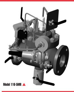
The Model 116-5MR opens and controls outlet pressure supplied into a deluge system when the solenoid valve is activated. After a fire event, the main valve must be locally reset using the ball valve manual reset lever on the deluge valve.
