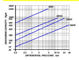
Cold water capacities are 2 to 4 times greater than the above . Safety factor = 1.2 - 1.5
