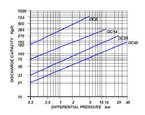
Cold water capacities are 2 to 4 times greater than the above . Safety factor = 1.2 - 1.5
