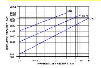
Cold water capacities are 2 to 4 times greater than the above . Safety factor = 1.2-1.5
