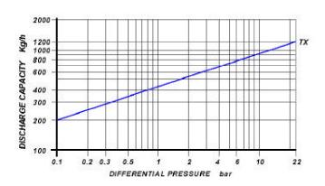
Cold water capacities are 2 to 4 times greater than the above . Safety factor = 1.2-1.5
