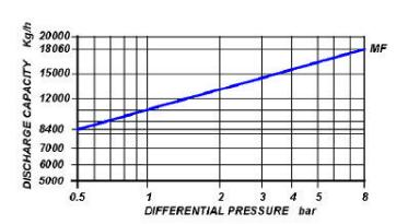
Cold water capacities are 2 to 4 times greater than the above . Safety factor = 1.2-1.5
