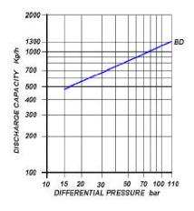
Cold water capacities are 2 to 4 times greater than the above . Safety factor = 1.2-1.5
