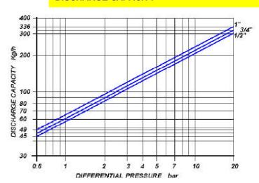
Cold water capacities are 2 to 4 times greater than the above . Safety factor = 1.2-1.5
