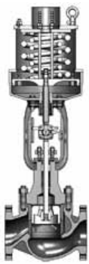
Low leakage pressure balanced cage type control valves
