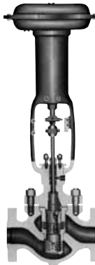
High pressure service low-noise cage type double seated control valve
