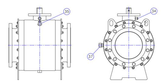
The S30T ball valve is equipped with grease injector on the neck for stem (34). And can be equipped on request with grease injector (37) on closure for the seals. With special ducts the grease gets to lubricate all moving parts. Grease fittings (37) are on the opposite side of bleeder valve so the operator can work in total safety.
